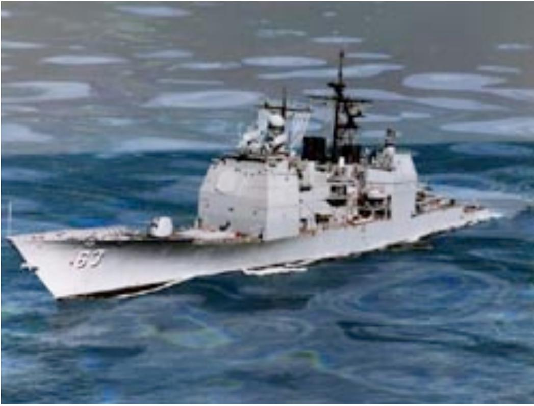
CG-63 has state-of-the-art technology. Her Mark 41 Vertical Launching System, SPY-1B Phased Array Radar, and Phalanx Close In Weapon System (CIWS) enable the USS Cowpens to fight threats from the air. Her
