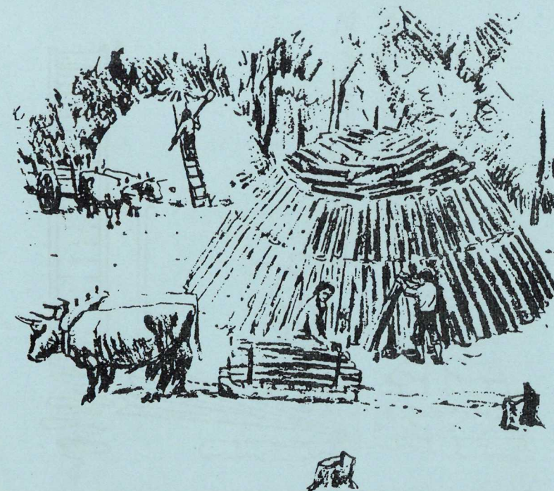
Green cord wood was stacked around the crow's nest to form a charcoal pit. Drawn by Joshua Tolford for Pioneer Iron Works by Mary Stetson Clarke.
