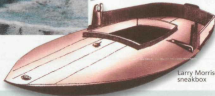
The Barnegat Bay sneakbox, designed by Hazelton Seamon in 1836, is a floating blind used by waterfowl hunters.
