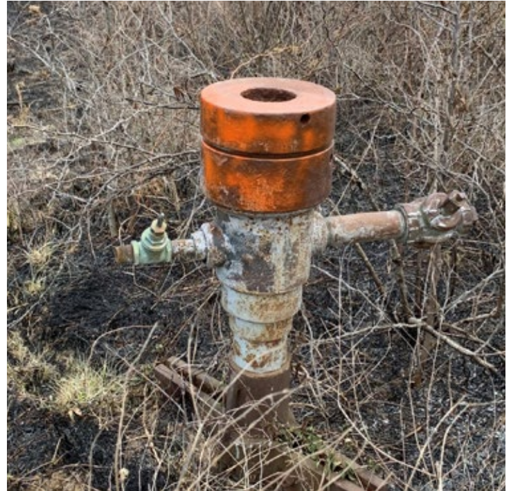
An orphaned oil well at Deep Fork National Wildlife Refuge in Oklahoma.
