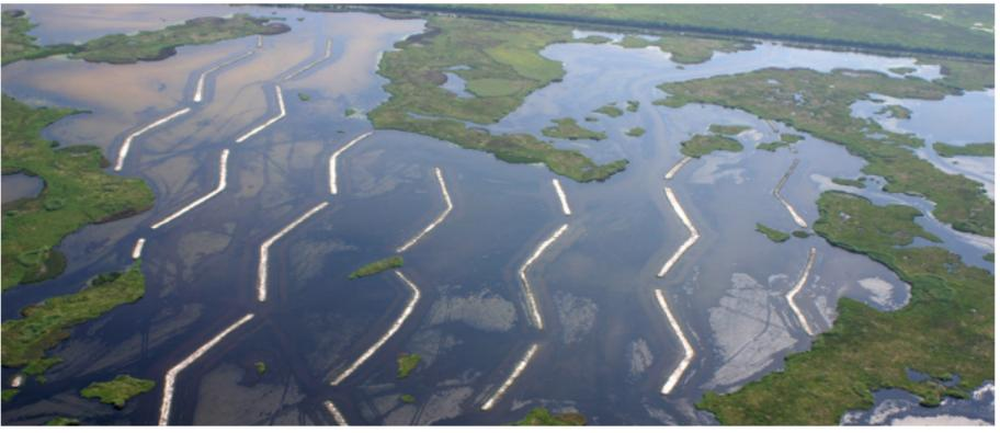
*Duck-wing shaped terraces reduce water turbulence and encourage plant growth.*
