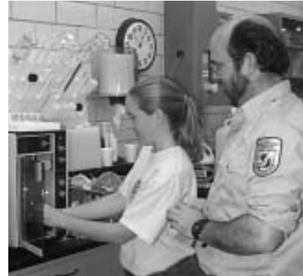
Jennifer Brownless, SCA student, learns to operate a Coulter Counter (a specialized piece of equipment used to analyze fish blood samples) under the guidance of Brian Hickson, fisheries biologist, at the Warm Springs regional Fisheries Center (GA).
