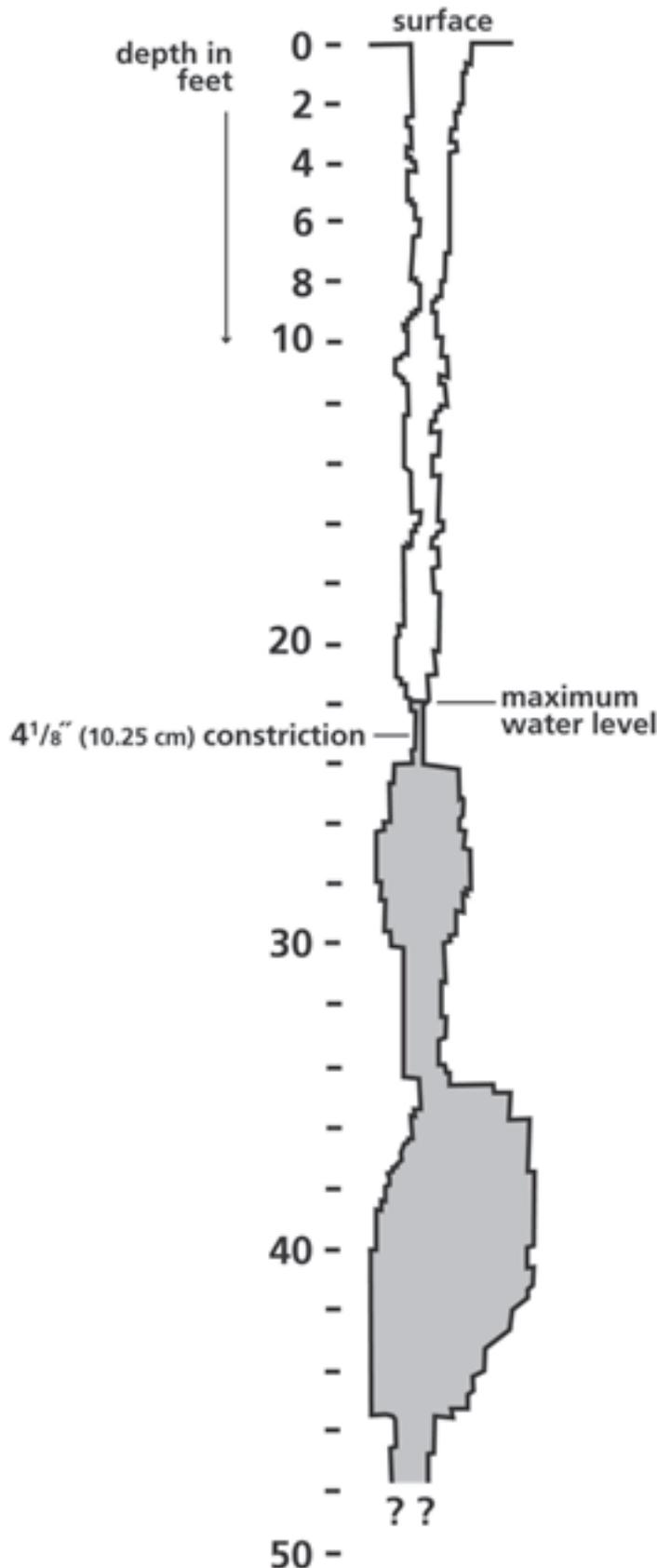
Geysers tubes or “plumbing systems” are not uniform in shape. They are usually crooked or constricted in many places. Measurements of Old Faithful’s conduit reveal a constriction at about 22 feet (6.7 m).
