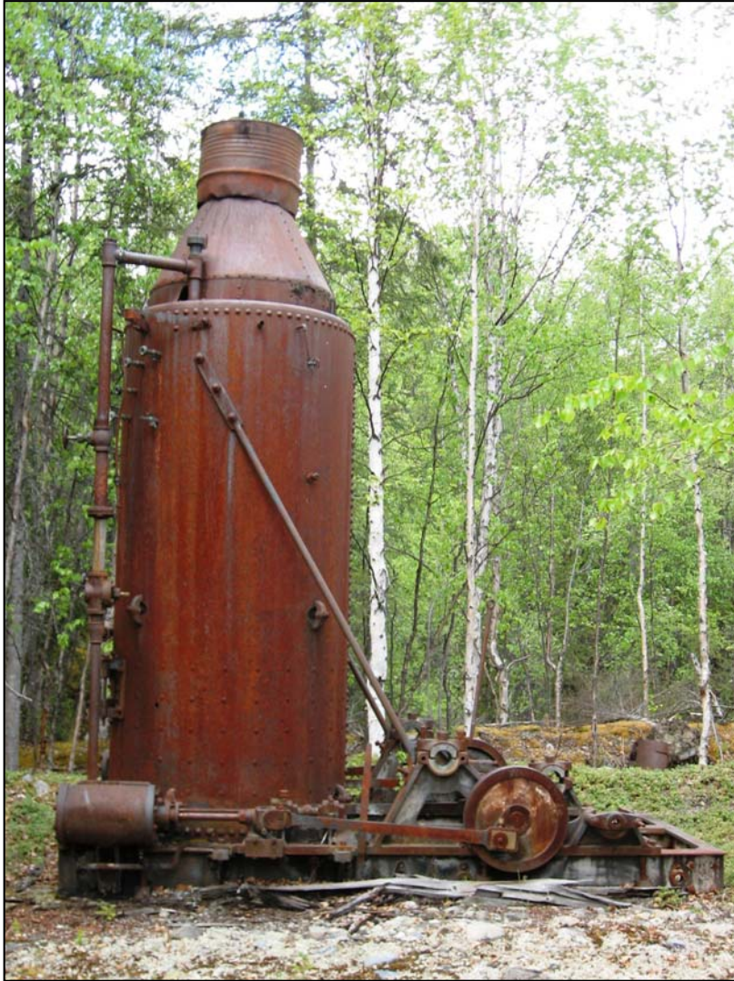
Imported by steamboat in 1911, this steam-powered “donkey engine” used cables to pull an excavator bucket, unearthing placer gold at Fourth of July Creek in today’s Yukon-Charley Rivers National Preserve.
