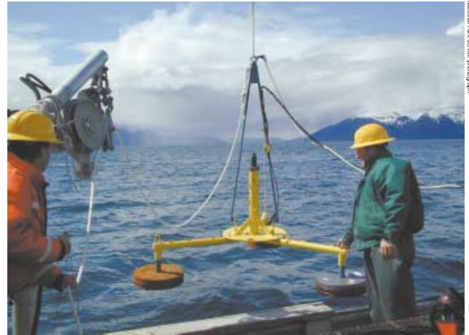
Installing the hydrophone, mounted on its customized aluminum anchor, near the mouth of Glacier Bay. The hydrophone anchor sits on the sea floor at 30 meters deep and is connected by a five-mile cable to a listening station at Park headquarters.
