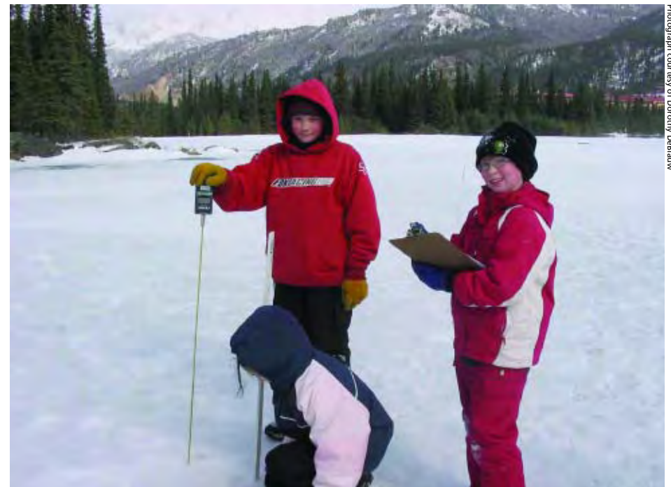
Figure 3: The snow depth is measured with a special probe. With a digital reader (on top of the probe) connected to a thermistor at the other end of the probe, the temperature on the ice surface at the bottom of the snow cover is measured.
