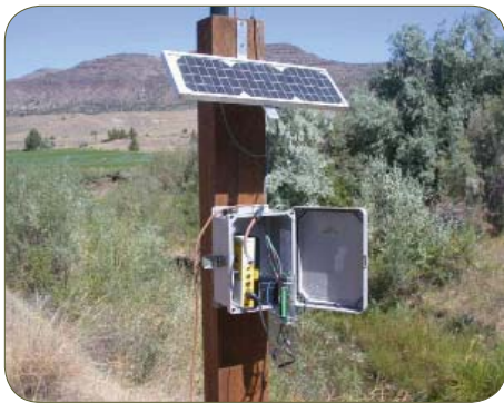
Bat detector used while monitoring bats at John Day Fossil Beds National Monument (JODA).
