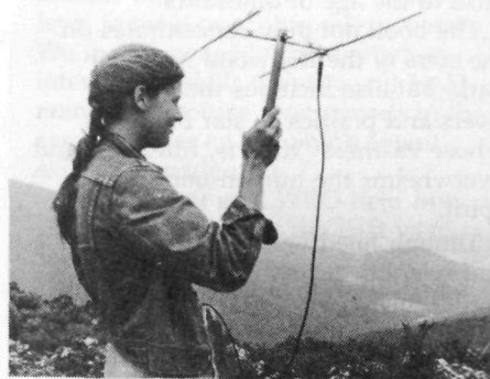
Alison Teetor turns the antenna until the signal comes in strongest on her radio receiver in the Shenandoah Bear Survey.
