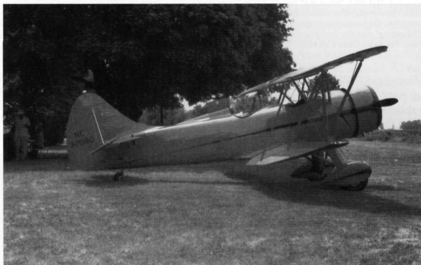
WACO UPF-7 NC 32080 is based in a small central Indiana airfield. Built in 1941, it shows a typical WACO design. Tubular metal struts and interior eliminated the need for elaborate cross bracing wires seen on earlier biplanes. Photo by Jerry Brown.
