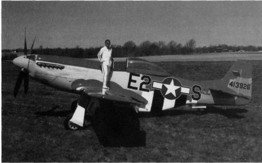
Significant design characteristics are often retained by military aircraft which never saw combat. North American P-51D 5NA "Mustang" No. 44-73436, for example, still retains its British designed Rolls-Royce "Merlin" power plant, as well as its "Laminar Flow" airfoil design. NACA (National Advisory Committee for Aeronautics, the precursor agency to NASA) scientists devised the airfoil which reduced drag by 50%, and the "Mustang" was the first practical application of this new airfoil type. This plane is based in northeast Indiana. Photo by Dean Cutshall.
