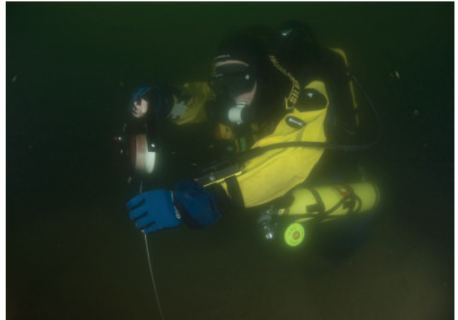
SRC's Dave Conlin deploys YSI sonde probe through the sands of the false bottom. NPS photo by Brett Seymour
