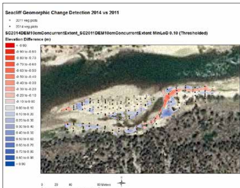
Figure 6. Plan view of the Seacliff sentinel site depicting spatial areas of erosion and deposition between 2011 and 2014. The figure was thresholded to only show differences greater than 10 cm. The figure indicates some deposition on the sand caps in the center of the site and mixed deposition and erosion at the downstream and upstream ends. River flow is from right to left in the image.
