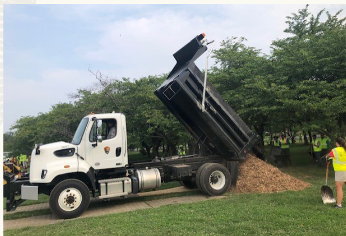
Wood chip mulch, created by the park from tree clippings, is dumped for workers to spread. Note: landscape mats are used to prevent damage to turf from equipment (NPS).
