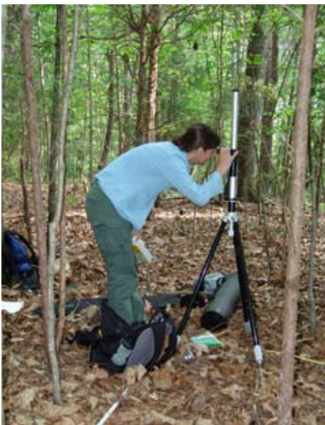
Kristina Callahan, Data Manager using the digital range finder to establish plot boundaries.
