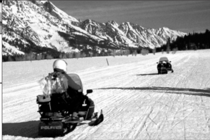
Figure 4. The study required a constant distance between the emitting snowmobile (front) and the trailing snowmobile that recorded the exhaust concentrations.
