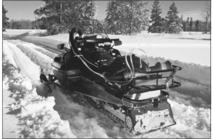
Figure 2. The study took place on flat terrain in Grand Teton National Park and involved a test snowmobile equipped for airflow measurement and exhaust sampling.
