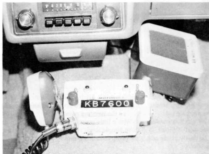
Fig. 1 Right: Telephone and external microphone remote controls for a base radio station. Fig. 2 Below: Control head, microphone and speaker for trunk-mounted mobile radio unit, and the mobile radio receiver and transmitter mounted in the trunk or luggage compartment of a vehicle.
