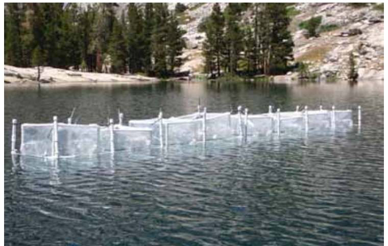
Limnocorral experimental setup in Sequoia National Park's Hamilton Lake to measure effects of different concentrations of nitrogen on algal growth. Photo: Andi Heard.
