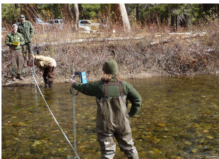
Taking streamflow measurements at Devils Postpile NM. Photo: Alice Chung-MacCoubrey.
