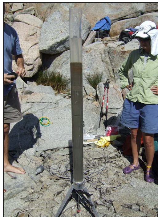
Example of a sediment core extracted from a Sierra Nevada lake. Cores are sliced into one-centimeter-thick segments and the chemical composition of each segment is analyzed to determine how lake chemistry has changed over long periods of time. Photo: Bob Meadows.
