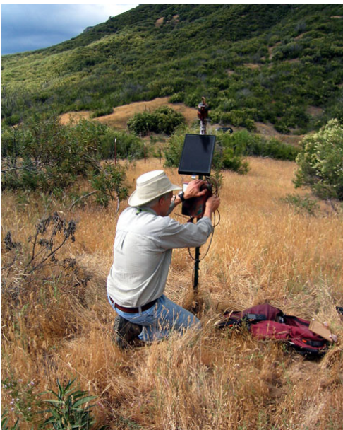
Bill Rainey setting up a bat detector to record bat calls. A solar panel charges the battery that powers the AnaBat detector, and bat calls are stored on a small memory card. Photo: Elizabeth Pierson.
