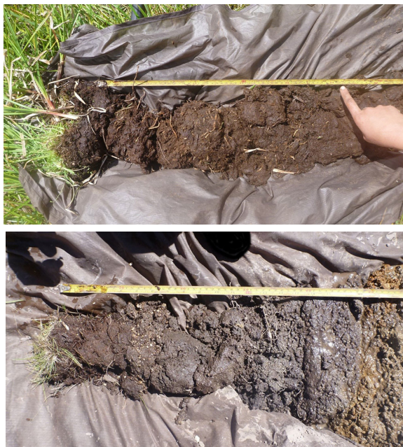
Upper photo is a fen soil profile with fragments of decayed vegetation. Lower photo is from a wet meadow, showing the gray and brown/yellow soil colors. NPS photos.
