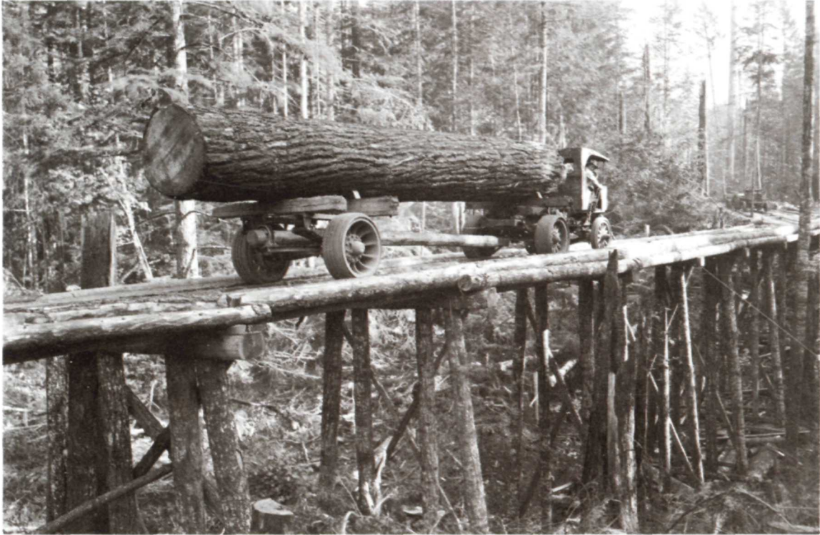
During the early years of the twentieth century, most logs—including the nine-foot-diameter fir below—moved out of the woods by rail. But by the 1920s trucks had appeared on the scene, and examples like the chain-drive, solid-tire model above heralded a new method of transport that would eventually supplant the more glamorous log train.
