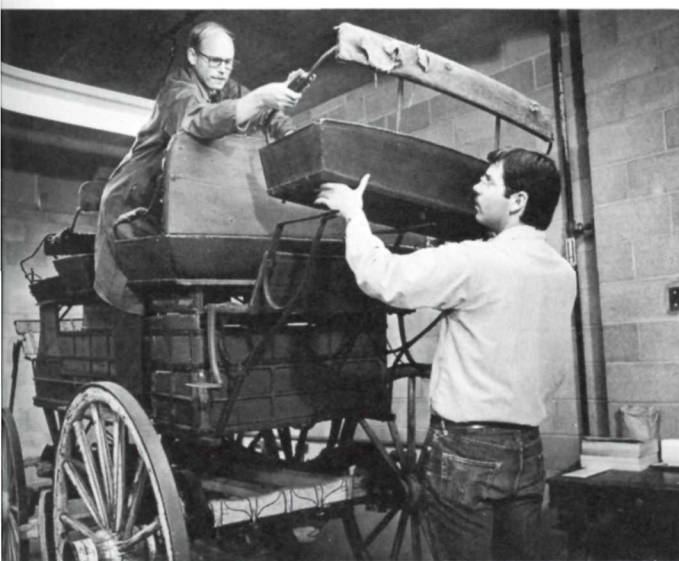
Removable seat of "convertible" passenger-freight wagon is extracted for repair. Seats out, the wagon hauled produce. Seats in, it carried people.
