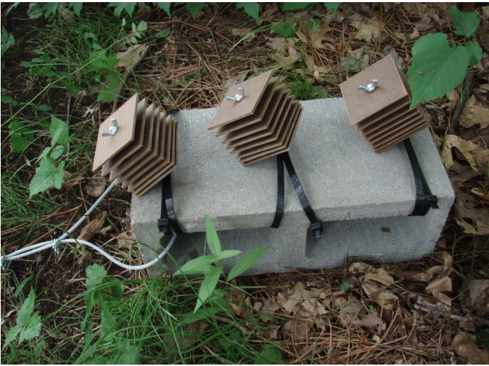
Hester-Dendy samplers are a series of wood tiles stacked together on a bolt and placed on or near the stream bottom. Insects colonize the tiles as they would a rock or log in the river. When collected, the tiles are each removed from the bolt and the attached insects are rinsed into a tray for sorting. NPS PHOTO
