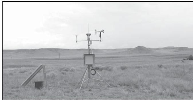
Portable ozone monitoring station with solar panels and battery box, in operation at Agate Fossil Beds National Monument, NE.
