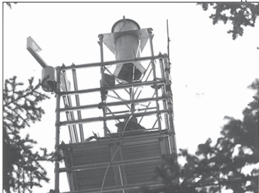
Figure 1. The deposition sampling tower at the Clingmans Dome monitoring site in Great Smoky Mountains National Park, TN, displays a particle volume monitor on the left and a cloud collector on the right.
