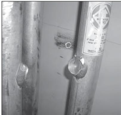
Figure 1. Crack at horizontal cross brace worsened to cause brace to come out.
