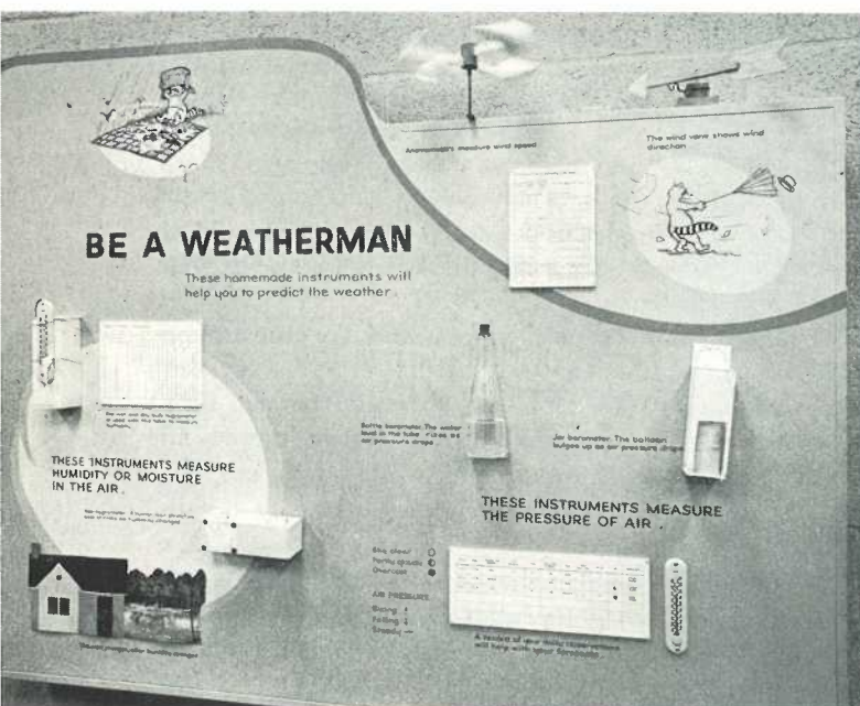
This display demonstrates how simple materials can be used to make weather instruments for home or classroom use. At the top a paper cup anemometer measures wind speed. Right, a milk carton barometer.
