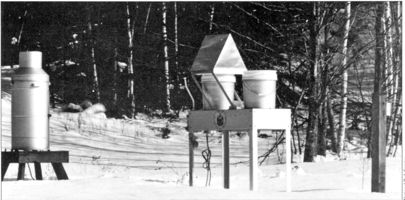
Acadia National Park monitors rain and snow year round. The cylinder on the left measures the amount and time of precipitation. The triangular roof on the right flips from bucket to bucket with each rain; the captured water is then tested for acidity.
