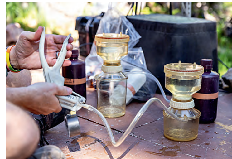
WEINMANN FILTERS water to measure chlorophyll so that the team can estimate the lake’s algae levels.
