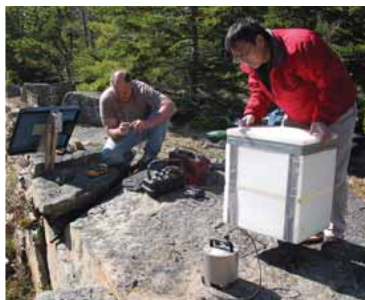
Seismic monitoring equipment being installed in the park.
