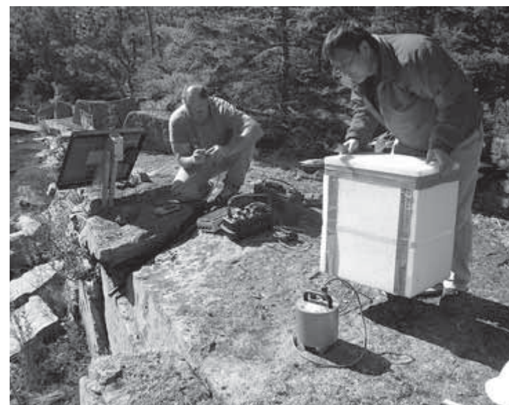
Seismic monitoring equipment being installed.
