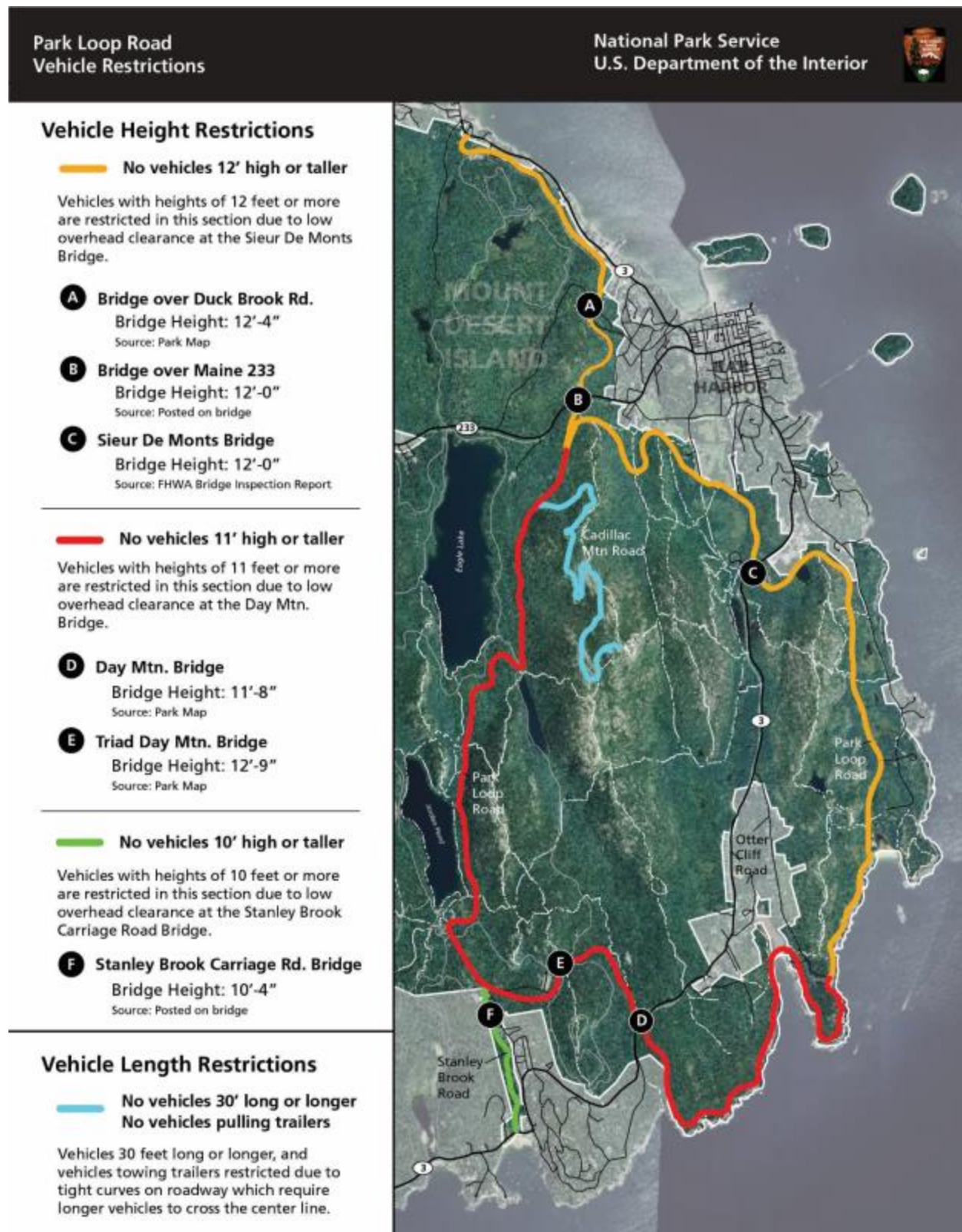
FIGURE 3. PARK LOOP ROAD GEOMETRY REQUIREMENTS
