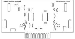
Dasibi 4-potentiometer electrometer board.
