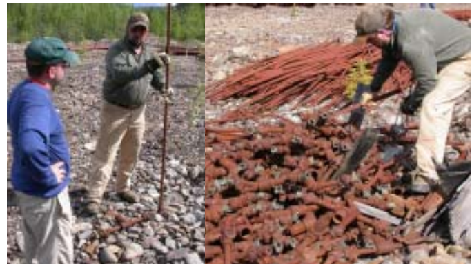
Right: NPS Historian Doug Beckstead holds a steam point which was used to thaw the permafrost ahead of dredging operations at the Coal Creek Historic Mining District in Yukon-Charley Rivers National Preserve. Burly young miners drove hundreds of these into the ground by hand. Standing next to Doug is Michigan Tech graduate student Larry Mishkar.
