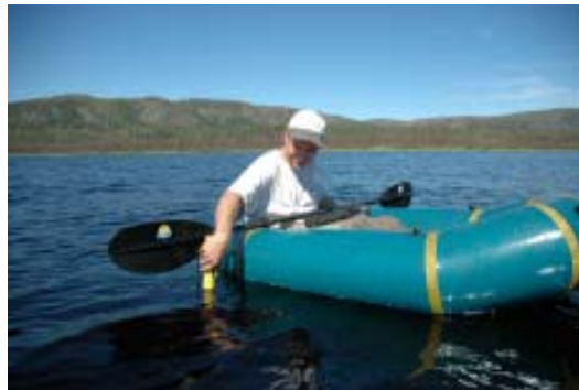
Doug Wilder, data manager for the Central Alaska Network inventory and monitoring program, measures lake depths to create a bathymetric map of the lake and track changes in lake water level.
