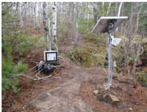
Real-time wave data and water temperatures are transmitted using wireless cellular technology to a host computer at UW-Madison.
