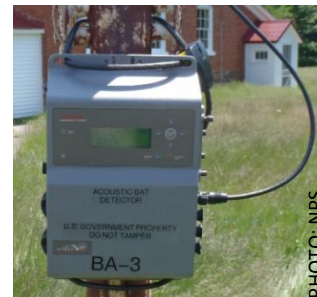
An SM3 unit deployed at Outer Island. There is a post elevating a microphone detecting the calls and occasionally an external power source found with each unit.
