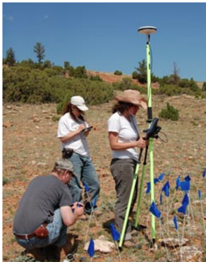
Students use GPS to locate and record each tipi stone and artifact.
