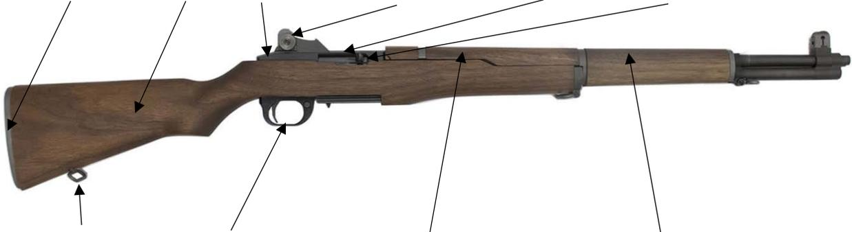
7. Butt Swivel. 8. Trigger Guard. 9. Rear Hand Guard. 10. Front Hand Guard.
