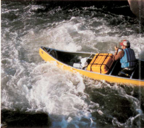
Whitewater canoes are especially designed without a keel so that they can be turned quickly. And they are made of materials that will not shatter or tear on impact.
