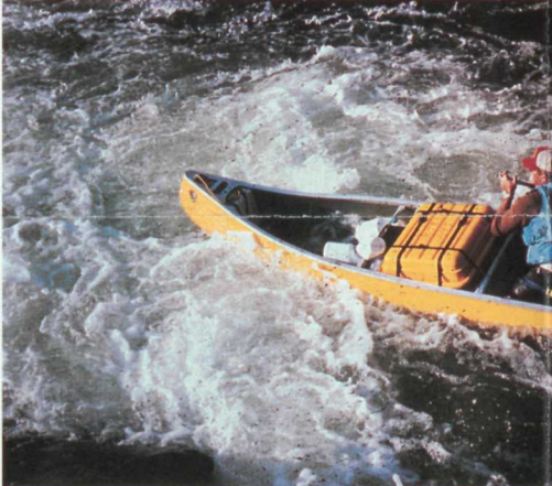
Whitewater canoes are especially designed without a keel so that they can be turned quickly. And they are made of materials that will not shatter or tear on impact.
