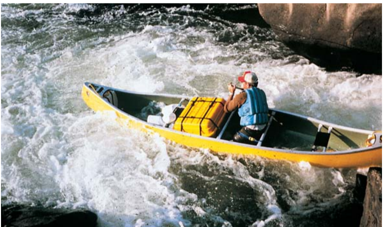
Whitewater canoes are designed without a keel so that they can be turned quickly. They are made of materials that will not shatter or tear on impact.
