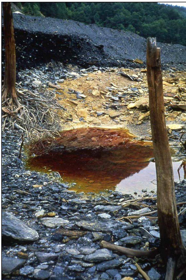
Figure 22. Ferric hydroxide byproducts shown at a coal mine at BISO. Known colloquially as yellow-boy, ferric hydroxide is a byproduct of acid mine drainage that can inhibit benthic production. [Source: NPS Photo]
