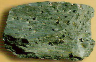
SCHIST: A dark, glittery rock that looks layered. A sheet-like mineral, mica, causes the sparkle. Sometimes distinct garnet crystals are found.
