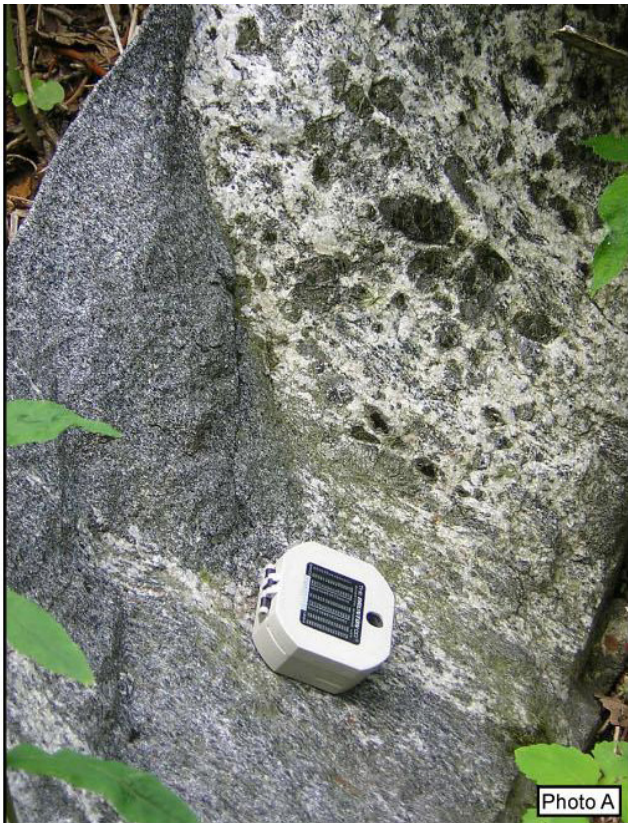
Figure 29. Photographs of mica-rich metagraywacke of the Ashe Metamorphic Suite. Biotite mica grains may be as large as a hand palm (Photo A). At outcrop scale, fractures in the rock pose a rockfall hazard. This outcrop occurs near the Little Pisgah tunnel. Graphic is part of photomosaic DMR-011 from Mersch et al. (2008a).
