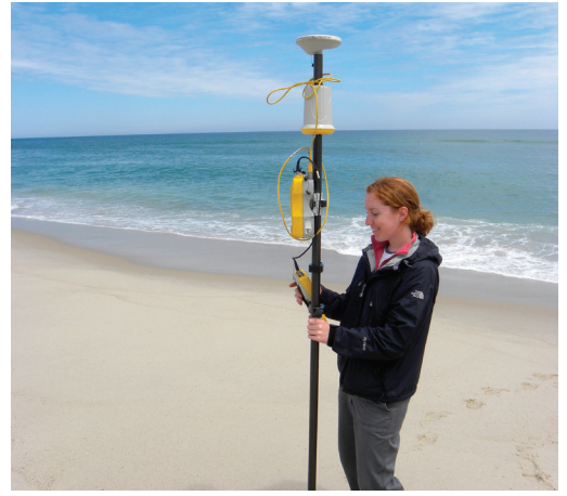
Collecting RTK GIS data for shoreline position monitoring
