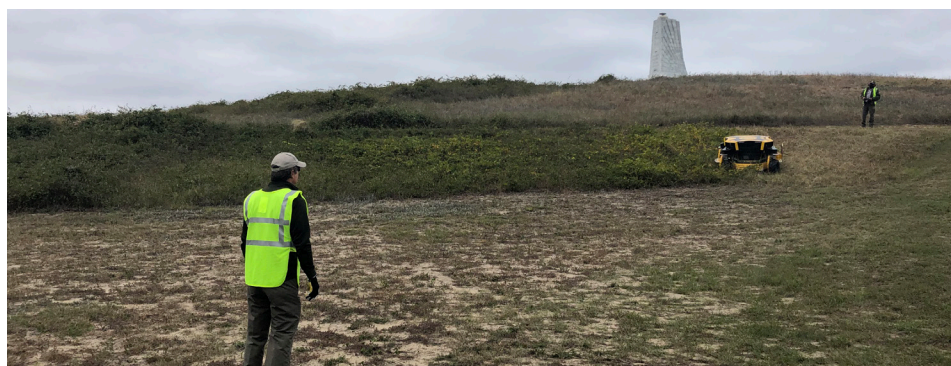
The remote-controlled mower easily cuts through thick brush and vines on the hillside.
