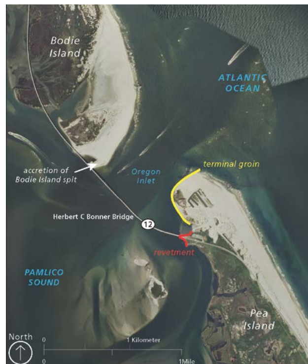
Figure 31. Aerial image of Oregon Inlet, stabilizing terminal groin and revetment, and erosion and accretion resulting from the hard stabilization. Aerial imagery from ESRI World Imagery base layer (accessed 23 July 2013), annotation by Jason Kenworthy (NPS Geologic Resources Division).
