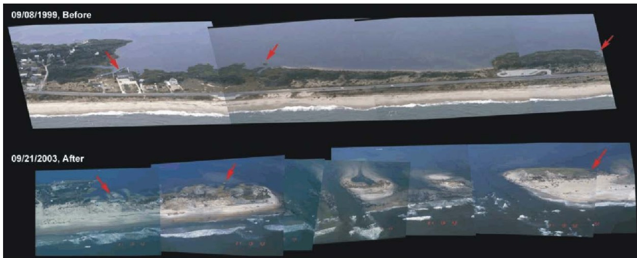
Figure 27. Inlet formation during Hurricane Isabel. Hurricane Isabel breached Hatteras Island in September 2003. The three-channel inlet was filled using dredged sand, and Highway 12 was rebuilt. The red arrows point to the same geographic locations on both oblique aerial photographs. This location remains vulnerable to future breaching. Figure 11 from Pendleton et al. (2004), created using US Geological Survey aerial photographs.
