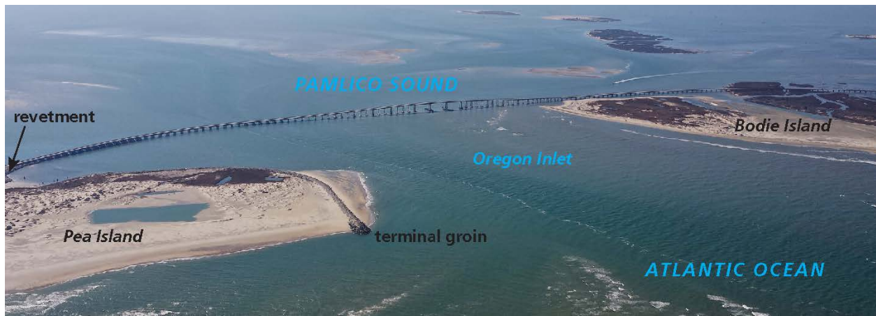
Figure 30. Oregon Inlet. The inlet was stabilized by a terminal groin and revetment to stop southward migration, which undermined the Pea Island Bridge onramp for Highway 12. Bonner Bridge is visible near the center of the photograph. National Park Service photograph taken February 2015, available online: https://www.flickr.com/photos/capehatterasnps/16217489383/ (accessed 27 April 2015).
