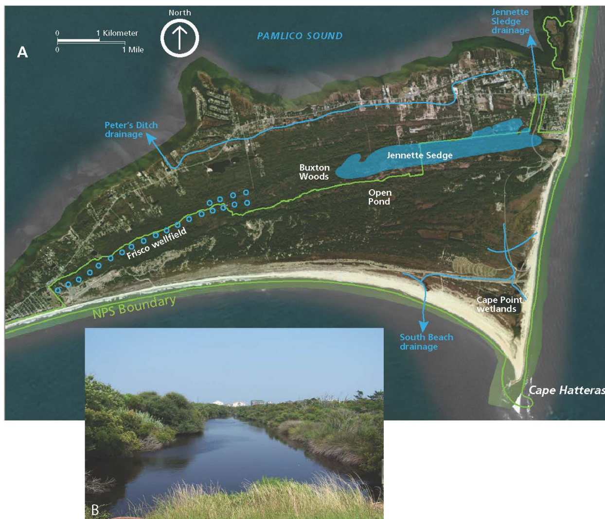
Figure 32. Drainage ditches near Cape Hatteras. A) Human -constructed drainage ditches affect water distribution and quality on Hatteras Island, and traffic crossing these ditches may contribute polycyclic aromatic hydrocarbons. ESRI World Imagery base layer (accessed 27 March 2014); annotation by Trista Thornberry-Ehrlich (Colorado State University). NPS boundary (2012; green line) courtesy Laura Pickens (Cape Hatteras National Seashore). B) Photograph of a ditch draining groundwater from Nags Head Village toward Pamlico Sound. Portions of Cape Hatteras National Seashore on South Bodie Island receive nutrients and microbial pathogens via septic leachate from the town of Nags Head and from the movement of groundwater through the sandy saturated soils into drainage ditches within the park. Photograph by Michael Mallin (University of North Carolina Wilmington) extracted from Mallin et al. (2006), plate 3.
